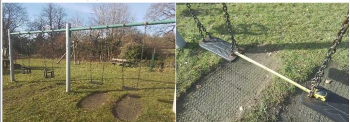
**Finding:** The seats are too close to each other as defined in **Action:** Monitor - No remedial work recommended BS EN 1176 Part 2; this is a low risk failure and no remedial action is required
